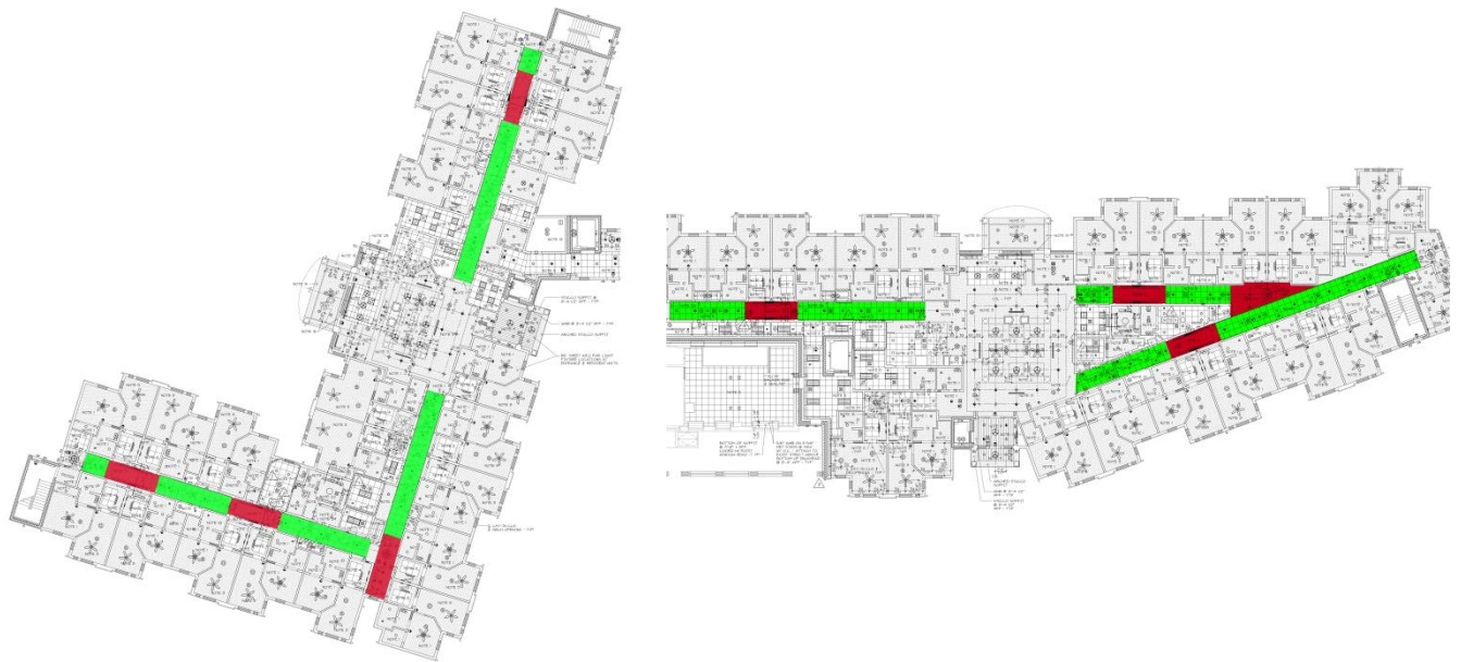
Figure 3.10 – Ceiling Heights West Wing (left) and East Wing (right)
